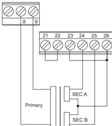
**Secondary to Secondary Ratiometric (S/S) Connections**
