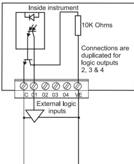
**Connecting to External Logic Inputs**
